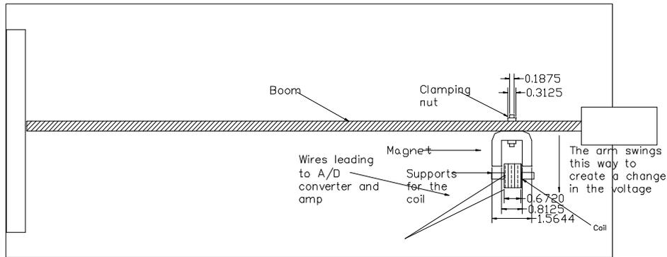
Figure 11: Magnet and Coil Assembly
